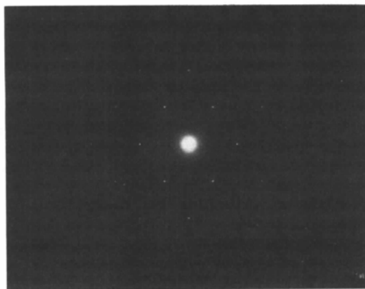
Fig. 4. Electron diffraction pattern ( hk0 ) from a solution-crystallized beeswax lamella. The pattern is characteristic of the orthorhombic perpendicular ( O_{\perp} ) methylene subcell.
